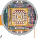
Silicon is an ideal material for integrated piezo-resistive resistors, which are often combined with the integration of signal conditioning. Especially at low pressures, these concepts can be provided at low cost. Silicon or MEMS (Micro-electromechanical systems) are very small and have a high sensitivity.
